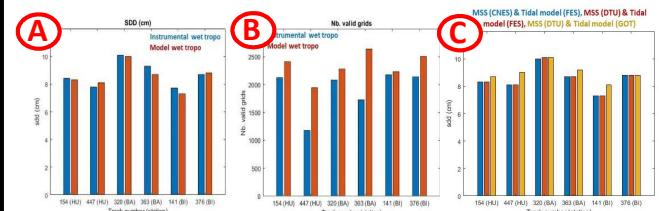
Average of the SDD (A) and number of valid grids (B) from the SWOT tracks analyzed at the three stations (HU, BA and BI). The SLA\_SWOT are estimated with the AMR (blue bars) and the ECMWF (red bars) wet tropospheric corrections.
