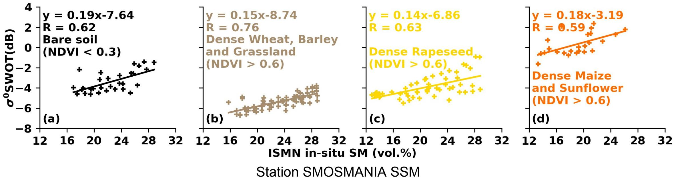
$\sigma^0_{\text{SWOT}}$  is correlated to *in situ* surface soil moisture with low and developed vegetation
