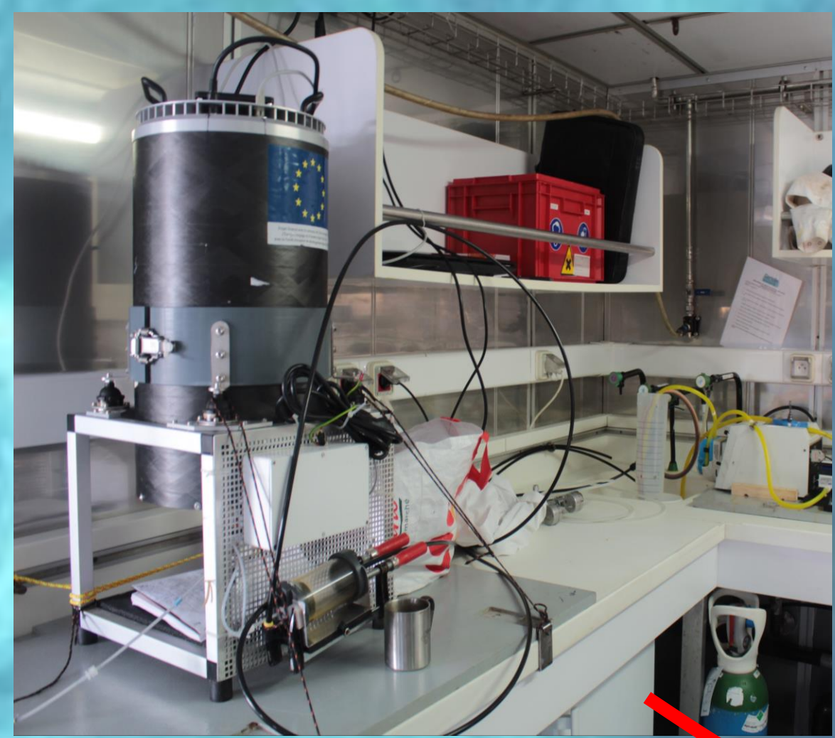
Automated flow cytometry (100 samples during 24h)
