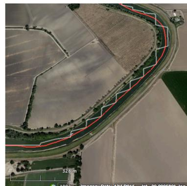
Centerlines are "fixed": they do not move pass-to-pass. They will be updated periodically (nominally yearly) Centerlines are computed starting from GRWL<sup>†</sup> and then adjusted based on composite low-flow pixel cloud.
