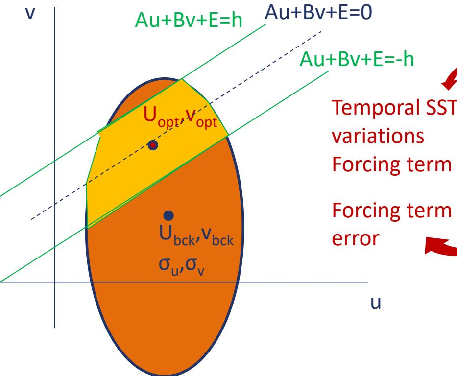
$q = \sqrt{(\sigma_u^2 \sin^2 \varphi + \sigma_v^2 \cos^2 \varphi)}$        $\varphi = \text{Arc tan}\left(-\frac{A}{B}\right)$
