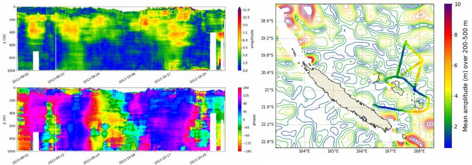
The geographic distribution of M2 internal tide (mean isopycnal displacement over 200-500 m) estimated from gliders is consistent with M2 tide estimated from altimetry (*Ray and Zaron, 2016*)
