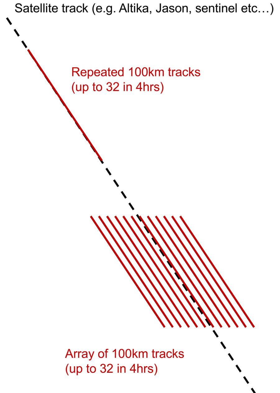
MASS lidar has a much smaller swath width than SWOT (~1km). Plan is to adjust the flight track depending on wave direction and wave period to avoid aliasing errors.
