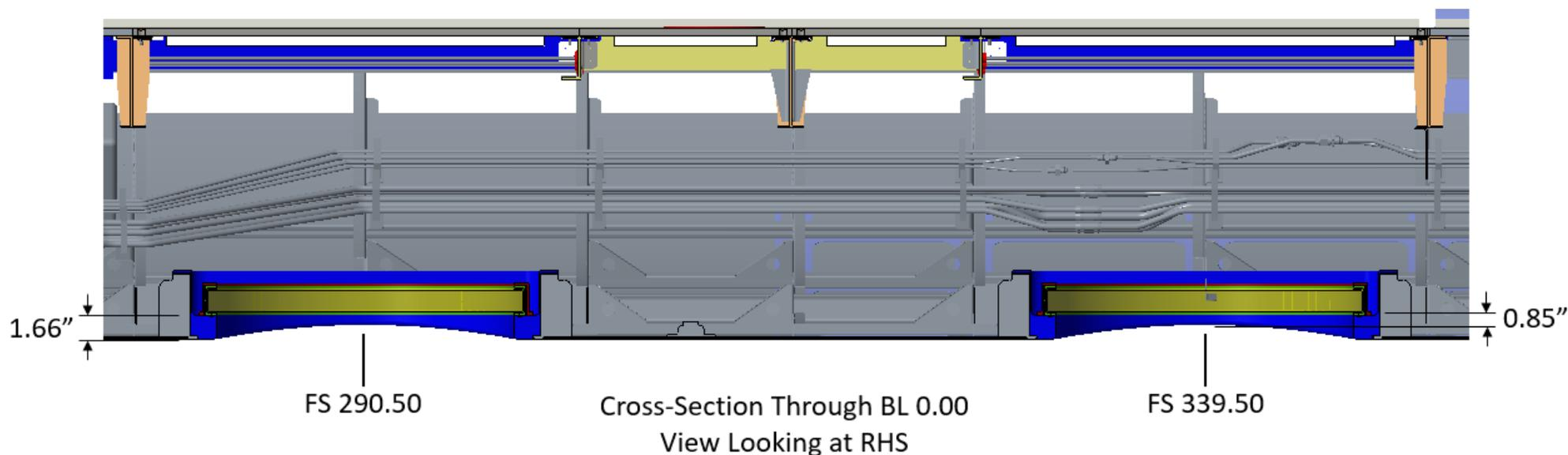
Need to design appropriate viewport window to accommodate all instrument wavelength requirements and ensure proper aircraft pressurization.
