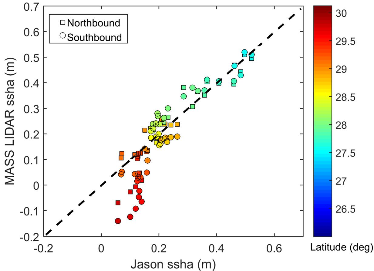
Fig. 7: Scatterplot of the SSHA measured by Jason-1 and the MASS lidar averaged over the along-track spatial resolution of the satellite for the latter. Note the divergence for the northern part of the track, as we get close to the continental shelf.
