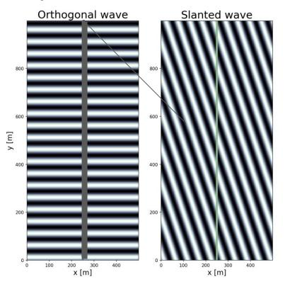
Across-track averaging lowers the wavenumber and attenuates the amplitude of oblique waves
