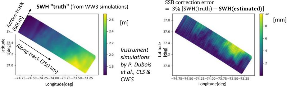
For SWOT, **SWH** is derived from **volumetric decorrelation** between the interferometric channels. ATBD currently plans 1 SWH estimate in the middle of each swath (+ nadir).
