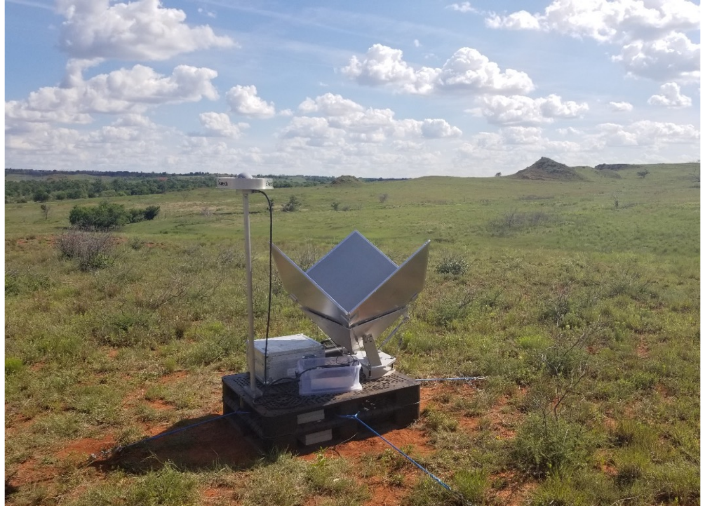
Site S02k pilot corner cube during GNSS metrology measurements
