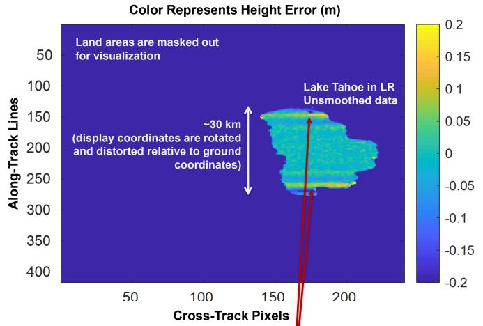
+/-0.2 m height errors due to processing artifacts (interpolator ringing) are evident
