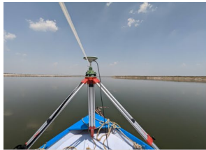
River WL GCPs using GNSS System
