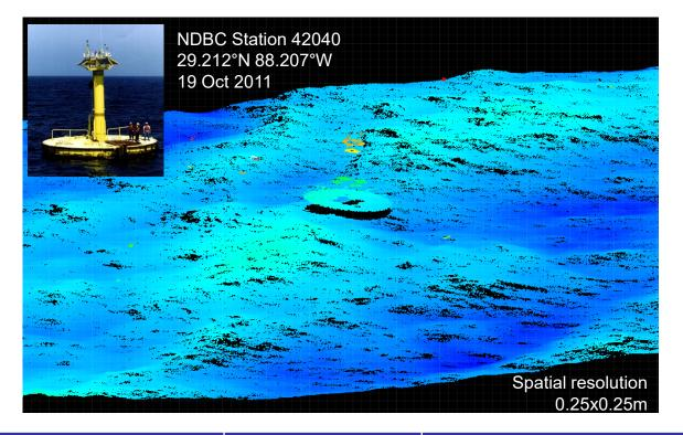
Example of surface elevation as measured from the MASS during a 2011 experiment in the Gulf of Mexico, flying above NDBC buoy #42040. (wind~12m/s, Hs = 3.1m, aircraft altitude = 500m AMSL)
