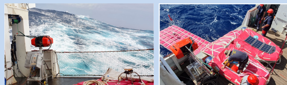
RapidCast (left) for CTD profiles in rough sea conditions and GPS blanket (right) to measure SSH onboard l'Antea © E. Kestenare
