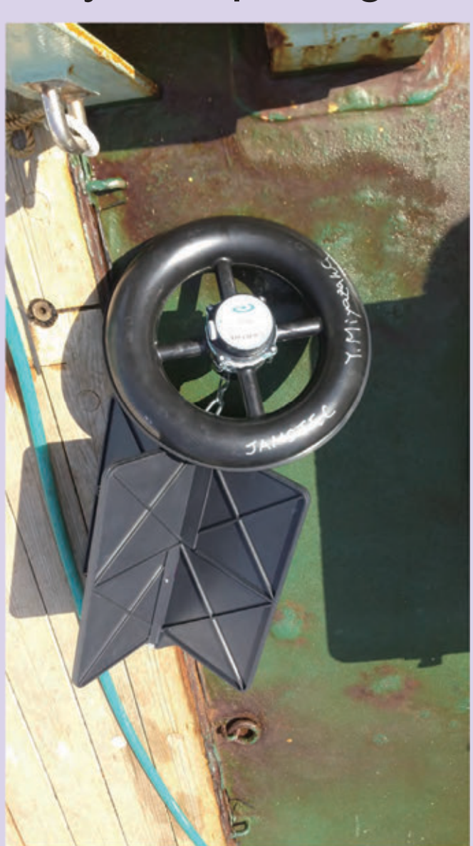
CARTE drifter Weight: 4kg Drogue depth: 40cm Telemetry: Microstar
