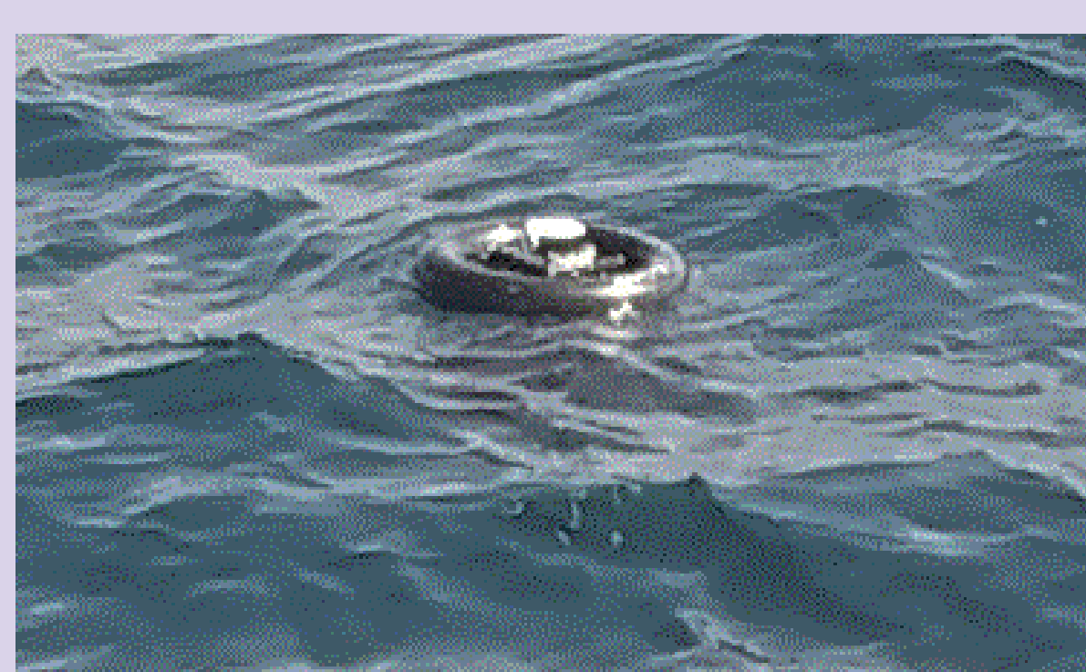
CARTE drifter Weight: 4kg Drogue depth: 40cm Telemetry: Microstar
