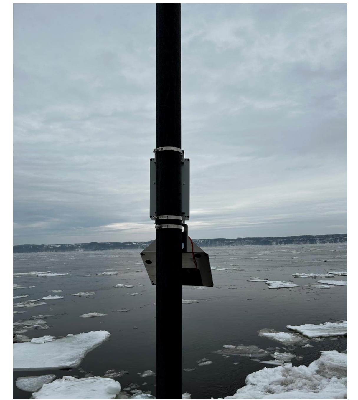
Figure 3: GNSS-IR sensor at Saint-Laurent-de-l'Île-d'Orléans.
