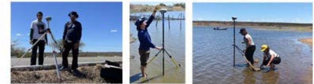
Absolute leveling / referencing of gauges with GNSS
