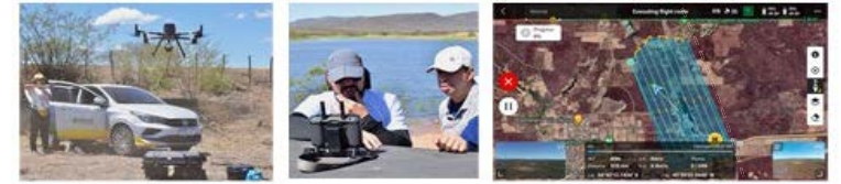
Drone Survey for High Resolution DEM and lake contour
