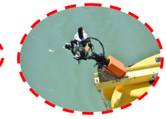
Cyclopée system : GNSS antenna/receiver and altimeter
