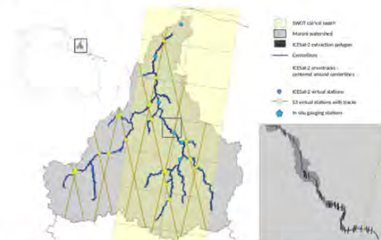
Hydraulic network (in blue) simulated with DassFlow 1D inflowed by MGB hydrological model (Paiva et al. 2013).
