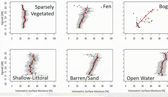
SWOT raster and pixel cloud products contain backscatter information that can be used to estimate surface moisture and vegetation structure.
